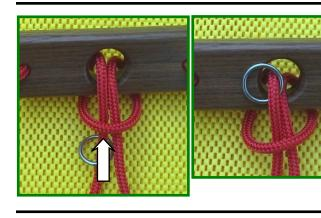
1: Give yourself a little slack in the rope and pass the ring under the loop so that it sits above the loop - Like so.....
